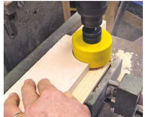
▲ Pic.10 A hole saw is gentler. The largest cutter wasn't large enough so it was set in a little, making the cut wider than a quadrant. This had the advantage of the central drill bit locating firmly in the ply rather than trying to hover on a corner. This cut was all but perfect. With a smaller cutter, Edward sawed the holes in the other leg components. Here, because the waste was not so readily ejected, the saw tended to scorch
